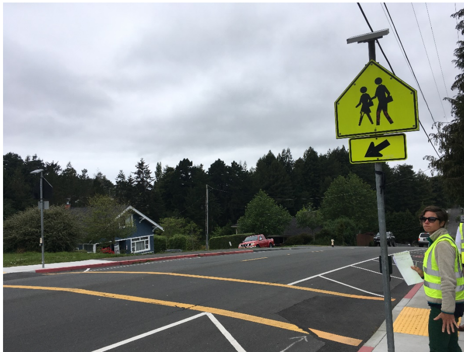
A workshop participant activates the solar-powered LED crosswalk sign in front of the school. No Parking Zones are marked on either side of the street. Photo Credit: California Walks
