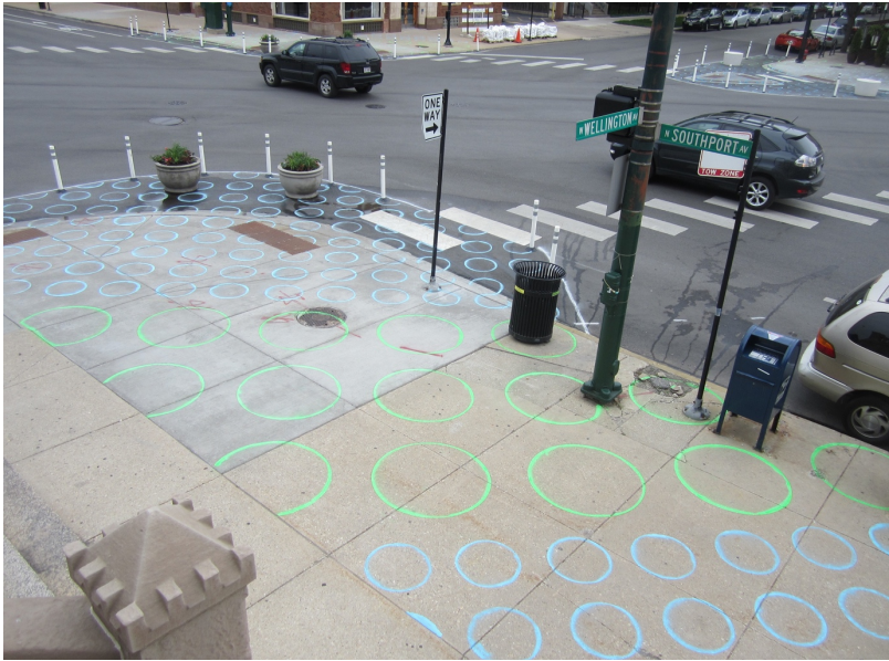
Example of a low-cost temporary curb extension that can be leveraged as a placemaking opportunity with art. Photo Credit: John Greenfield.
